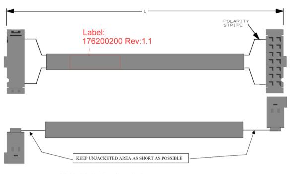
2540-14 (w Strain relief) Ribbon Cable is not wrap under Strain relief.
